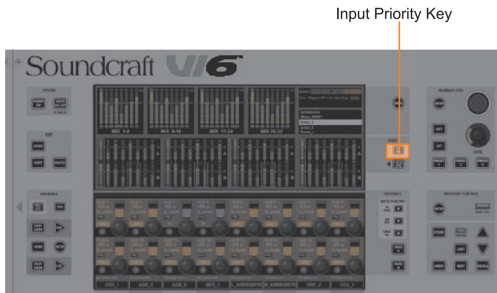
Figure 11-10: INPUT PRIORITY Key
