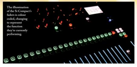
Looking at the 'IN A' layer for the moment, inputs 1-22 are controlled by the faders, and each channel has other dedicated indicators and switches: in the space directly above each fader are selector buttons for solo, 'on' (which is, in effect, a mute switch) and a select button which links that channel to the detailed channel controls within the 'strip' above.
