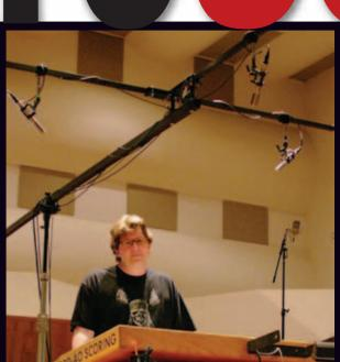
PIRATED SOUNDS: Alan Meyerson stands at the conductor's position on the scoring stage at Todd-AO during the tracking of the score for Pirates of the Caribbean: Dead Man's Chest. Over Meyerson's head is a unique Decca Tree approach employing Royer R-122V vacuum-tube ribbon microphones. A total of 255 tracks were laid down to two **Digidesign Pro Tools** HD systems and mixed on a Euphonix System 5 console. See story on page 24.
