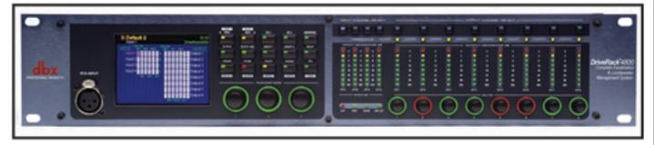
left mid, right mid, left hi, right hi. For those of us raised on English analog crossovers, it's a simple task to make the outputs Sub, Low, Mid, Hi, Sub, Low, Mid, Hi without affecting the linking of PEQ filters and other inserts within the software. Clever.
