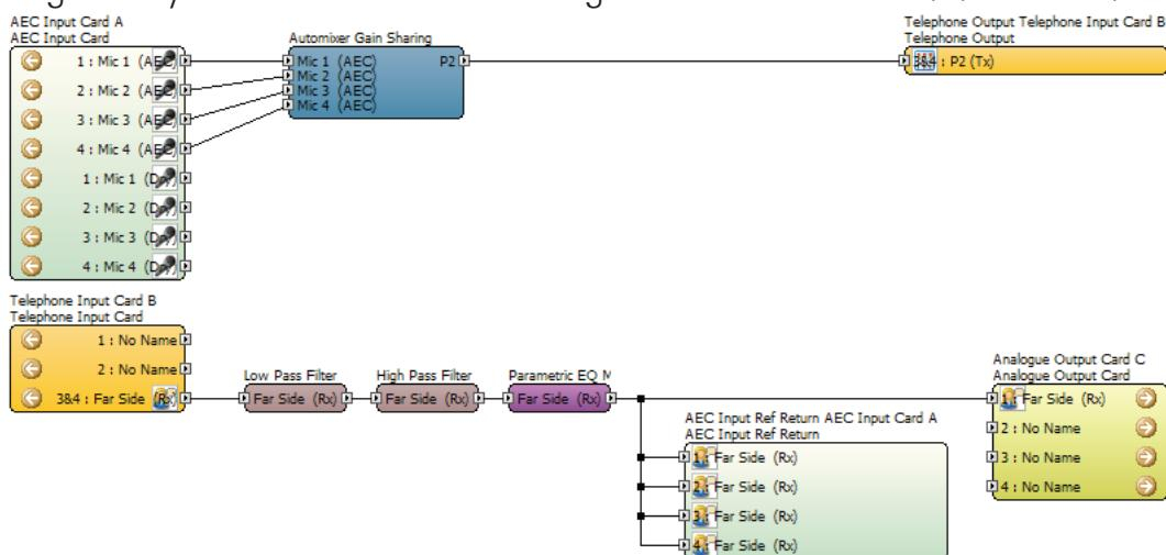
The image below is the same design with the Reference signal wired incorrectly. Because the Reference is taken before the room processing blocks, the AEC algorithm will not understand that certain frequencies were cut/boosted intentionally and will not be able to model the room to its full ability.
