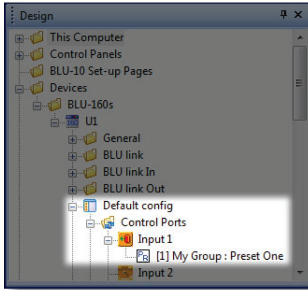
The Control Ports in the Design Tree is updated to reflect the Direct Action assignment. When the Configuration is loaded to the device, the Parameter Preset will be recalled when the Control Input pin is shorted with the Common pin.
