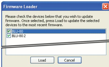
This will display a list of all the Soundweb London devices discovered on the network. Make sure all the devices listed are checked and press the Load button. The firmware transfer will take several minutes, during which time the devices may reboot several times.
