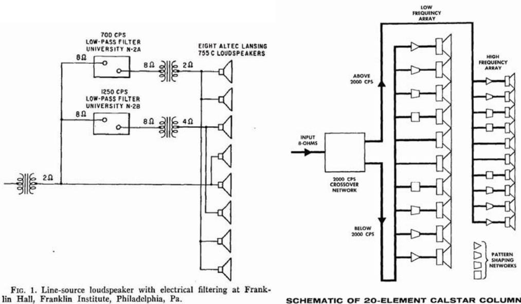
**Figure 1. From Klepper and Steele<sup>1</sup> shows a simple network for improving directivity control and Novak<sup>2</sup> (on the right) shows more complex filtering**
