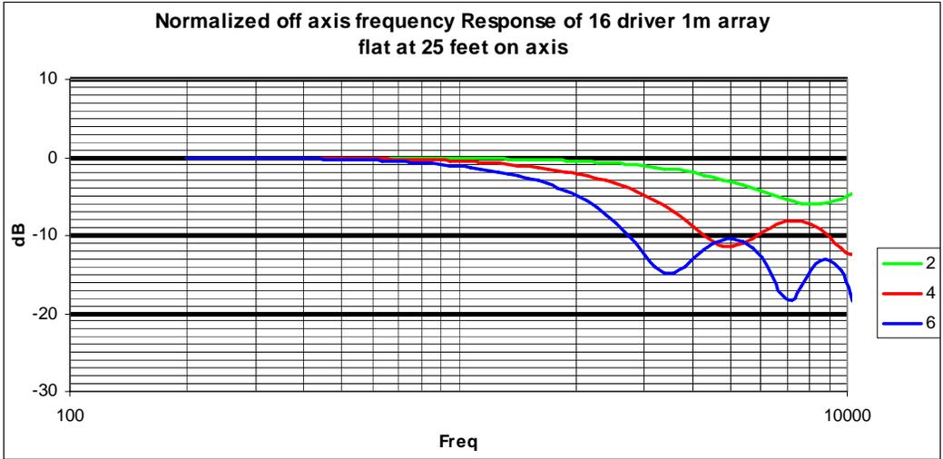
Off axis response at 25 ft 2, 4 and 6 degrees off axis. Response changes radically within a very small forward beam.
