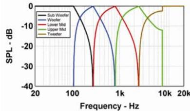
Fig. 16. Crossover frequency responses for the example five-way constant-beamwidth speaker system shown in Fig. 15. The response exhibits critical frequencies (pointed tops) at 119 Hz, 297 Hz, 825 Hz, and 2.475 kHz; and crossover frequencies (-6 dB) of 160 Hz, 408 Hz, 1.15 kHz, and 3.72 kHz. Above 7.4 kHz, the tweeter operates on its own with full drive. Below 119 Hz, the subwoofers operate alone at full drive.
