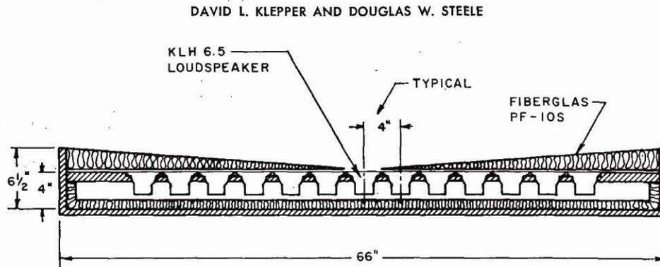
FIG. 4. Section through line-source loudspeaker (enclosure is made of  $\frac{3}{4}$  in plywood).
