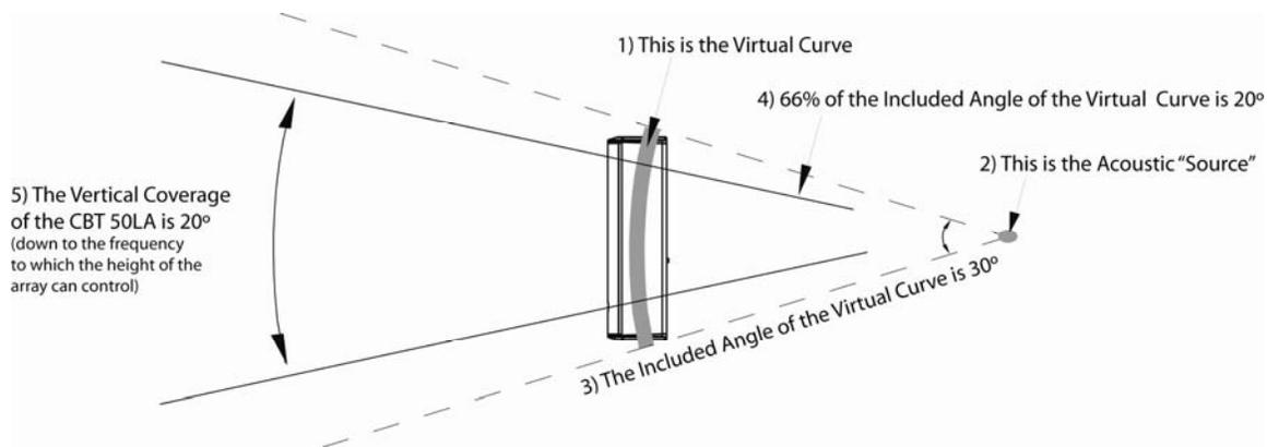
**Figure 8. A virtual curved array can be achieved by bending it with time delay. The apparent point source is behind the array.**
