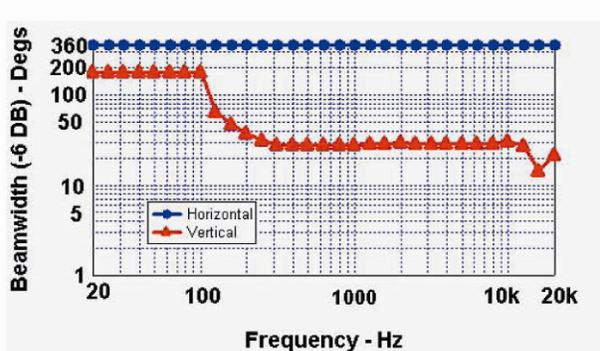
Fig. 80. Farfield above-ground-plane beamwidth (-6 dB) versus frequency for Legendre-shaded 50-point 1.25m-high 45° delay-curved straight-line source located on a ground plane (Fig. 79). Horizontal: blue circles. Vertical: red triangles.
