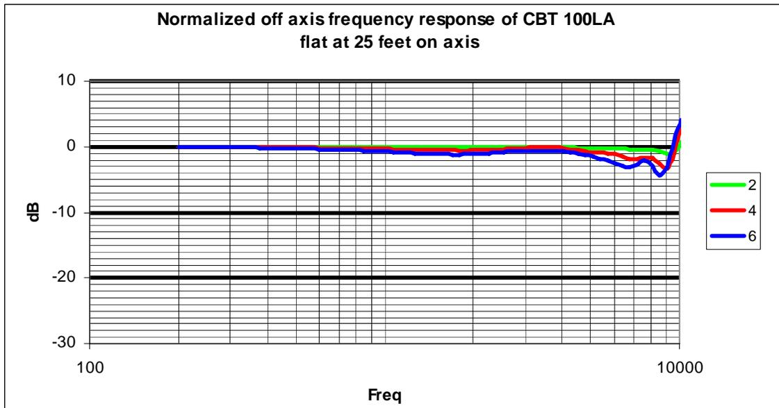
Off axis response at 25 ft 2, 4 and 6 degrees off axis. Unlike the straight array from figure 5 the CBT 100LA response is very consistent on and off axis.
