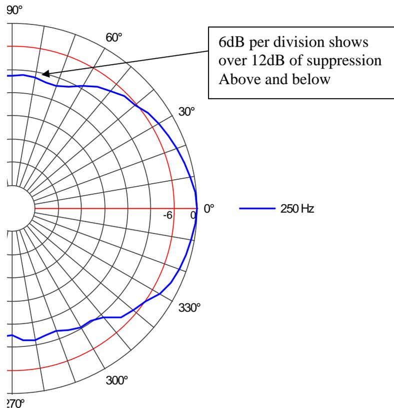
**Figure 17. The vertical polar of the CBT J and CBT 70JE coupled together at 250 Hz. Even though the pair is specified as having pattern control down to 400 Hz there is still well over 12dB of suppression above and below the array at 250 Hz.**
