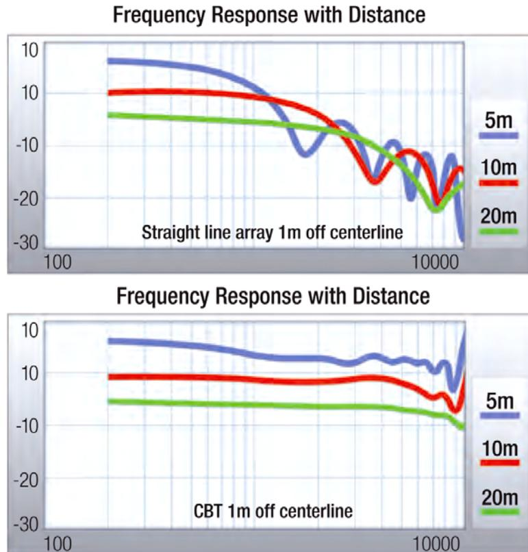
**Figure 19. The simulated response of a 1m straight line array and JBL CBT 100LA with the microphone just 1m off the centerline of the speaker.**
