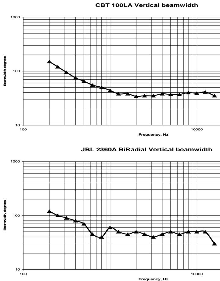
**Figure 10. The constant directivity capability of the CBT 100LA can be seen as compared to a large JBL BiRadial horn with even smoother and more consistent pattern control. The vertical pattern control of the CBT 100LA is nearly identical to the large cinema horn from the cinema industry standard JBL 4675.**
