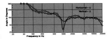
Figure 3. Directivity vs. Frequency (4430)
