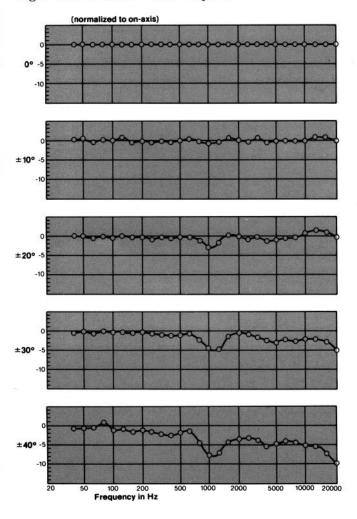
Figure 5. Vertical Off-axis Response (normalize to on-axis)
