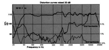
Figure 16. Distortion vs. Frequency (4435)
