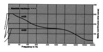
Figure 12. Maximum Continuous Output
