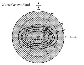
2 kHz octave bandwidth constant sound pressure contours. Same conditions as 500 Hz contours. This data may be considered essentially the same as would be observed at 4 kHz and 8 kHz, considering only the -3, -6, and -9 dB isobars.
