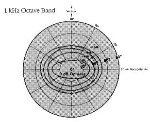
1 kHz octave bandwidth constant sound pressure contours. Same conditions as 500 Hz contours.
