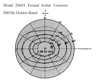
500 Hz octave bandwidth constant sound pressure contours of 0 to -12 dB in steps of -3 dB. The contours are plotted on polar grid lines with on axis being the center of the plot. The data was gathered by taking an octave polar plot at all oblique angles from 0° (horizontal) to 90° (vertical) in steps of 5°
