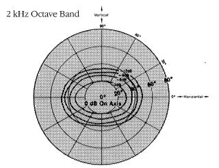
$2~\rm kHz$  octave bandwidth constant sound pressure contours. Same conditions as 500 Hz contours. This data may be considered essentially the same as would be observed at 4 kHz and 8 kHz, considering only the - 3, - 6, and - 9 dB isobars.
