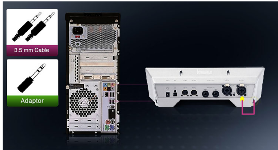
External A.I. Loopback Test
