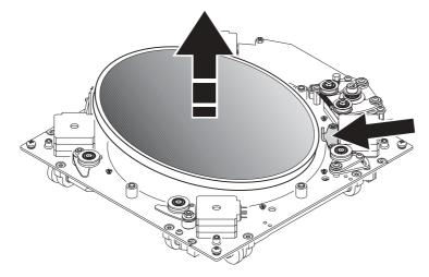
10 Place the replacement lens into position in the chassis (J) being careful to avoid the rotation stop bracket (marked with an arrow in the following illustration).
