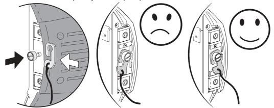
6 Push the barndoor unit into place so that the interface connector on the rotation assembly (at the rear of the barndoor unit) connects correctly to its counterpart on the MAC 2000 Wash. Ensure that the cable slack is taken up *outside* of the barndoor unit.
