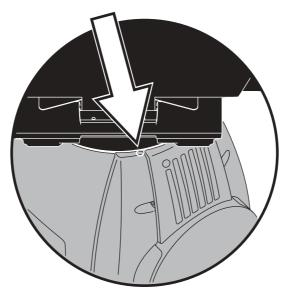
7 Hook the fold of safety-wire slack under the lip of the MAC 2000 Wash head cover as shown in the following illustration.
