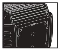
4 If present, remove the lens that is installed on the MAC 2000 Wash by unscrewing the four quarter-turn screws, pulling the lens housing away from the fixture, and releasing the safety cable.
