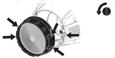
5 Attach the barndoor safety cable to the MAC 2000 Wash and lock it in place using the thumb-screw. Ensure that the cable slack is kept away from the optical path.
