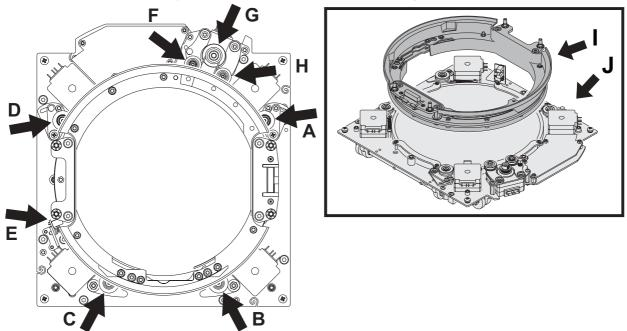
4 Move the rotation assembly (I) to a position where it is free of the sensor at position E.
