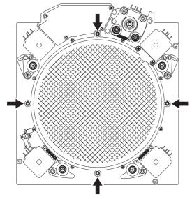
11 Install the four plates the hold the lens against the chassis (J) by pushing up on the spring-loaded bolts and sliding the plates into position against the rubber-coated posts (indicated with an arrow in the following illustration).
