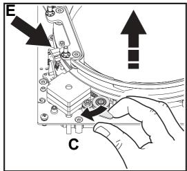
8 The lens is held in place in the chassis (J) by four plates. To release each plate, push the sprung bolts from underneath the lens chassis. This will release the pressure on the plates and allow you to pull them free.
