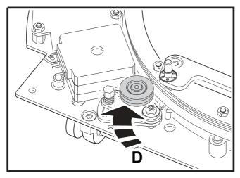
17 Push the roller (not the spring-loaded bolt) at position F until it is locked into position.
