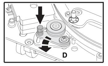
6 Release the roller at position F by pressing down on the spring-loaded bolt
