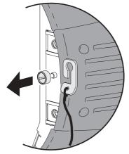
8 Do not operate the MAC 2000 Wash without a front lens or barndoors installed. If installing one of the standard lenses, attach the safety wire and place the lens on the fixture. Lock it into place using the 4 quarter-turn screws.
