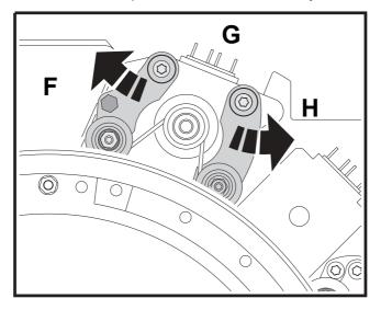
14 Ensure that the rotation assembly (I) is free of the sensor at position D.
