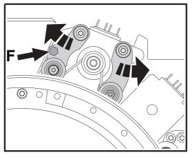
7 Pull back on the spring-loaded clamp at position C and lift the rotation assembly (I) clear of the lens chassis (J), being careful to avoid the sensor at position E, and carefully freeing the rubber drive belt from the rollers at positions F, G and H.
