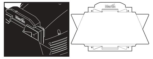
5 Open the barndoor blades to an angle sufficient to access the four recessed quarter-turn screws with a flat head screwdriver.
