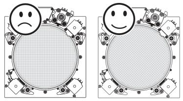
The lens should sit snugly against the four rubber-encased posts marked in the following illustration.
