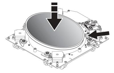
*Note* If you are installing the standard diffuser lens, the textured side should face the lamp and the rotation assembly.
