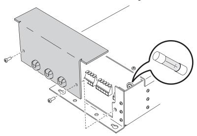
2 Remove the three cable glands from the holes in the cable-terminal access cover.
