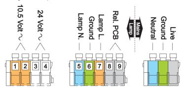
5 Clamp the respective leads into position on the terminal blocks. Note that the other ends of two of the cables will be connected to corresponding colorcoded terminals in the Imager luminare's junction box. Therefore it might be a good idea to make a note of the terminal block color/wire color combinations to ensure that they match when connecting the cables to the Imager luminaire.
