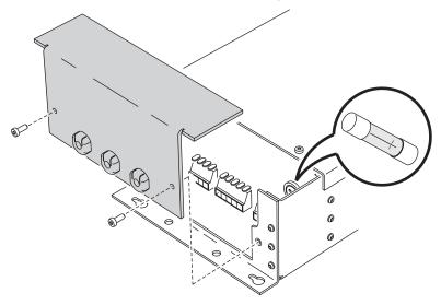
3 Open the fuse holder using a small flat-head screwdriver.
