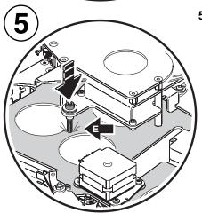
5. See left. Fully tighten the Allen screw in the filter-holder. The screw will press against plate E. The frost filter is now installed.
