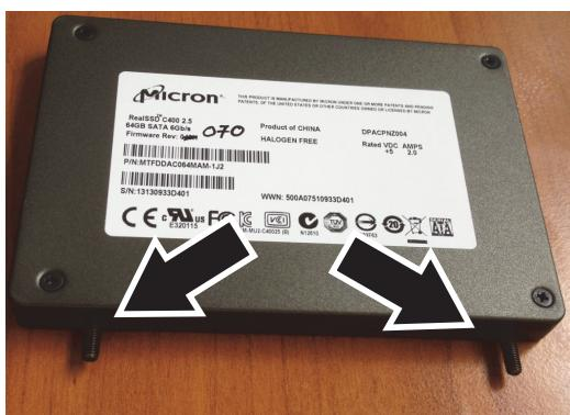
8. Unscrew both hard disk screws (arrowed) using a Torx T-10 driver and gently lift and pull out the hard disk. Disconnect the SATA cable and DC power cable from the hard disk.
