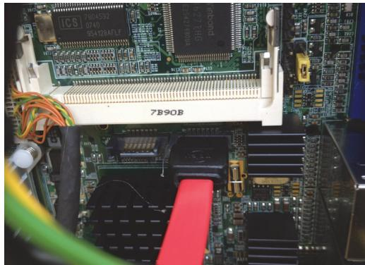
12. The SATA cable is glued into its connector on the mainboard. Taking care not to damage the PCB and other components, disconnect and remove the SATA cable.
