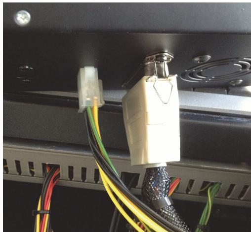
3. Place the Cerebrum module gently on top of the Programmer module, then disconnect the Power and Centronics Data cable from the Cerebrum Module.
