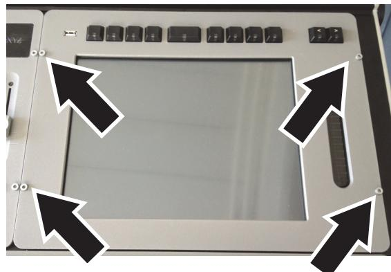
2. Unscrew the 4 screws that hold the Cerebrum in the frame. Use Allen key N° 6 (3 mm).
