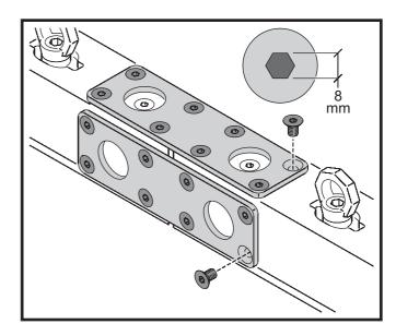
Figure 6: Joining Plates for Header Connection Brackets
