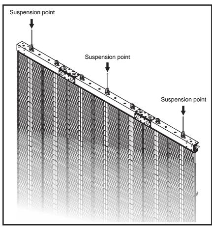
Figure 7: Installation 7 panels wide
