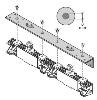
Figure 5: Header Connection Bracket (Double Header illustrated)
