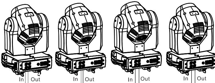
The number of daisy-chained fixtures is limited by the number of DMX channels required by the fixtures in relation to the maximum 512 channels available in one DMX universe. Note that if independent control of a fixture is required, it must have its own DMX channels. Fixtures that are required to behave identically can share the same DMX address and channels. To add more fixtures or groups of fixtures when the above limit is reached, add a DMX universe and another daisy-chained link.
