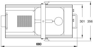
Figure 1: Dimensions in mm
