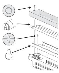
3 Using a Phillips screwdriver, loosen the two screws holding the cover of the wiring housing in place; remove the cover.
