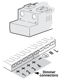
there are fewer connectors on Cyclo models with fewer than four tubes.) Connect the ground (earth) lead to the - terminal. Connect the other leads to the appropriate connectors. Notes that there are two connectors at each position and that you can use either one of these.
