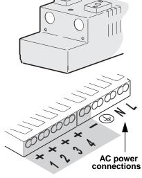
Use the three terminals *not* shaded in grey to connect AC power - L live, or positive), N (neutral) and ground (or earth).
