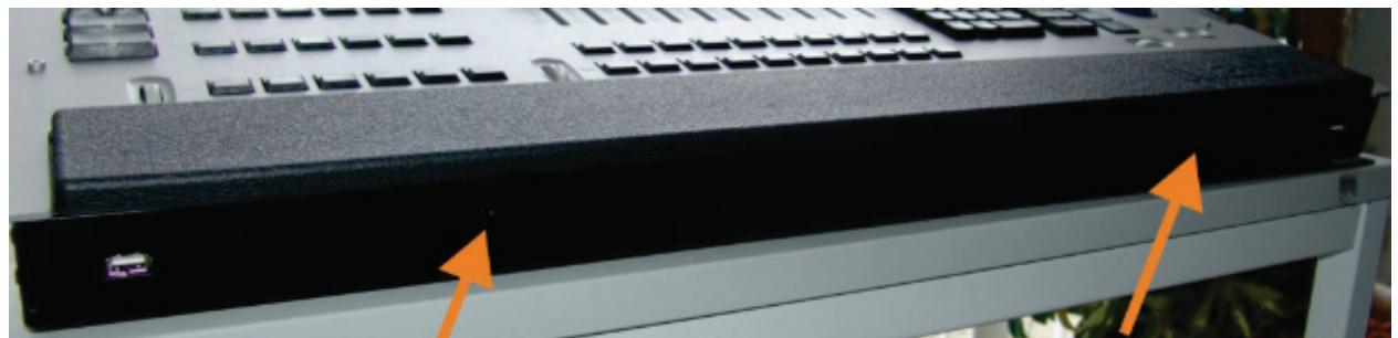
Two T20 screws below the hand rest on the front
