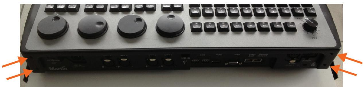
Four T20 screws on the back
