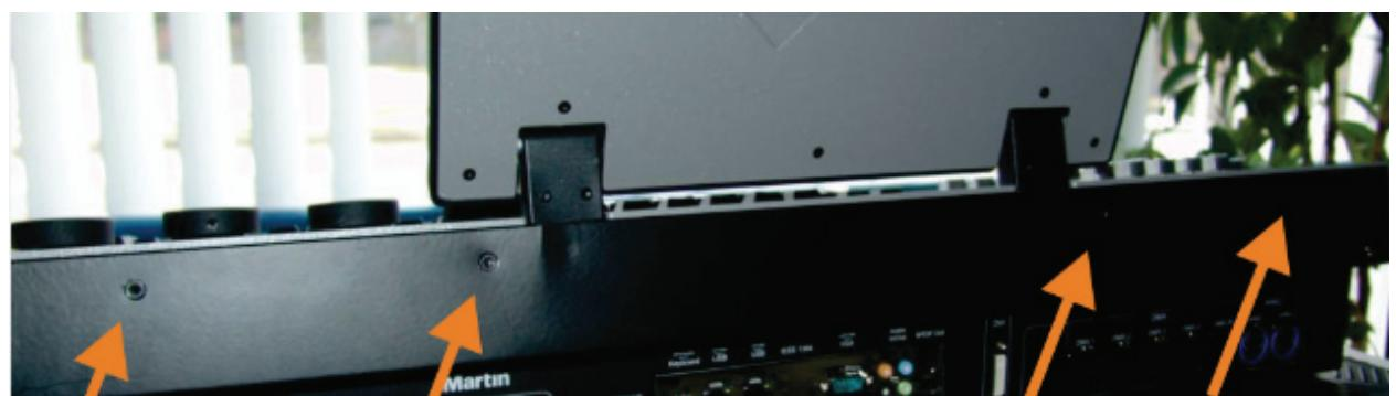
Four T20 screws on the back
