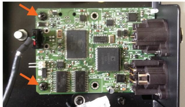
**Four XLR Torx screws, LEDs and 2 T10 Torx screws.**
