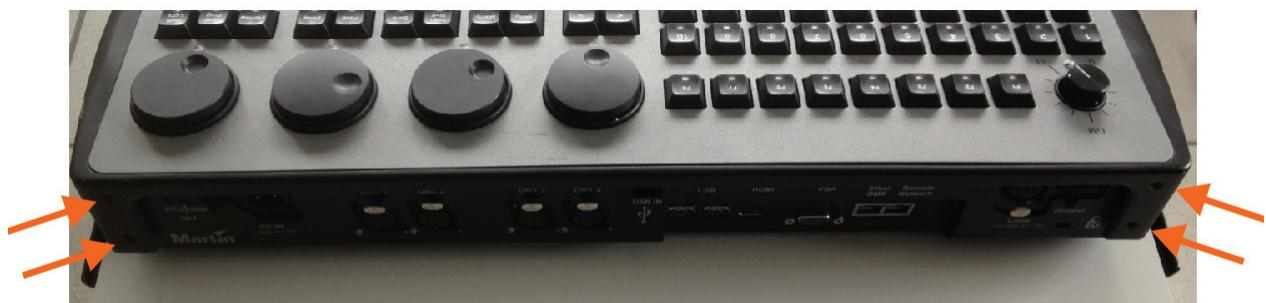
Four T20 screws on the back
