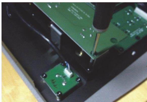
4. Remove the 6 Torx T10 screws and lock washers, and keep them for re-use.
