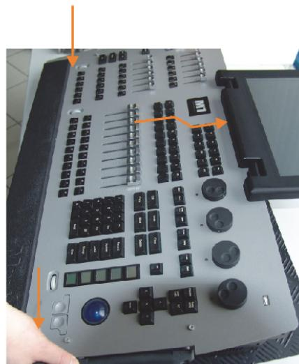
3. Guide the top plate back into its position carefully underneath the screen housing and lower it into the chassis. If it is difficult to fit at the back, hold it with one hand and hold the screen housing with the other. A slight pull backwards on the screen housing will open more room for the top plate to settle into place.
