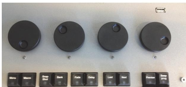
11. Flip the front panel and place the new encoder knobs onto their shafts.
