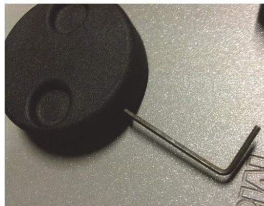
1. Using a 1.5 mm Allen key, release and remove the 4 encoder knobs.
