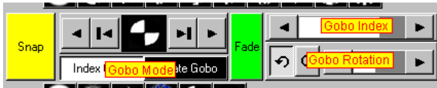
MAC500/Roboscan 918 Rotating gobo controls.
