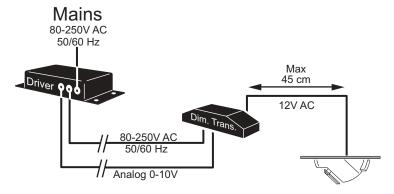
Using the Oracle controller, or a DMX control device, it is possible to dim, and power on and off the Alien 05s via the intensity channel.
