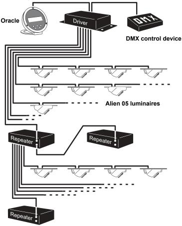
Warning: Do not mix Alien 05 luminaries and 05 Repeaters on the same Output link. Connect only Alien 05 luminaires, or only a 05 Repeater, to an individual connector. This applies to both the 05 Driver and the 05 Repeater.
