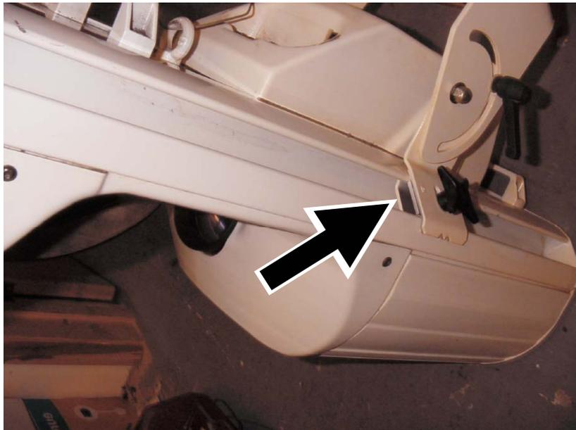
**RoboScan 918 Pro mounting bracket clamp plate (arrowed)**
