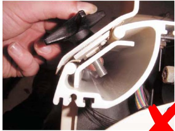
**WRONG – Warning! Do NOT install the clamp plate this way around**
