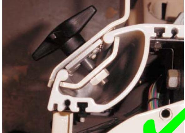
**RIGHT – Install the clamp plate this way around**
