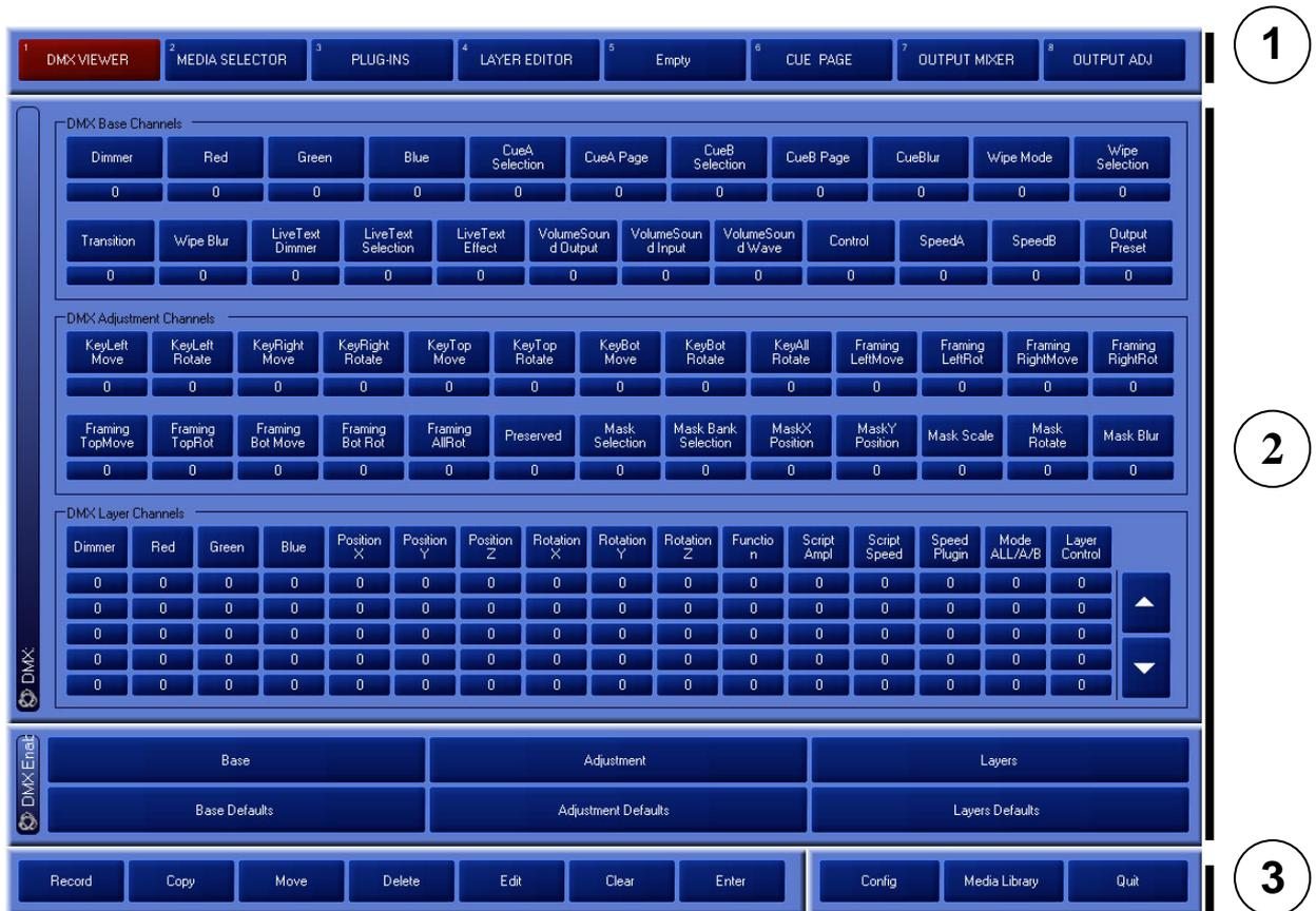
The Maxedia's Graphical User Interface (GUI) consists of three main parts (see illustration above):
