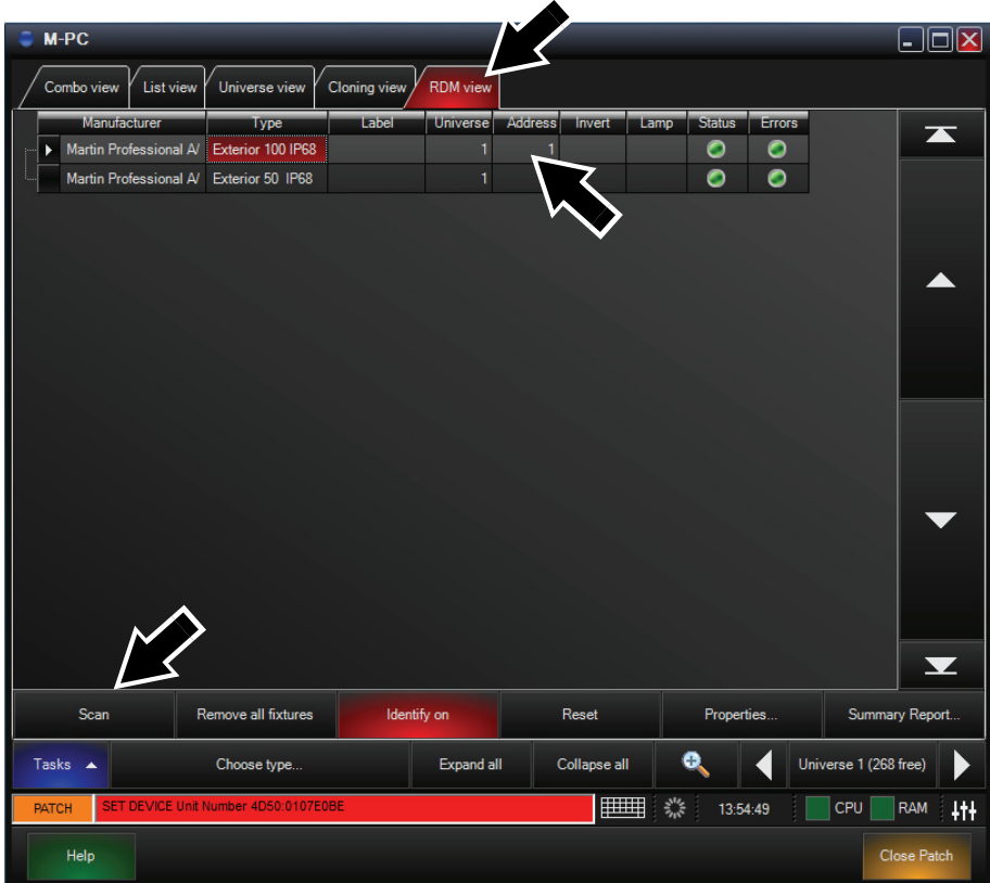
Figure 38: M-PC RDM View
