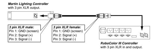
DMX CONTROLLER: Most DMX controllers have 5-pin XLR sockets for data output. Use a 5-pin to 3-pin phase-reversing adaptor, such as P/N 11820003, as shown below. This adaptor connects pin 2 on one end to pin 3 on the other end, and vice versa, to correct the difference in polarity between the RoboColor III system and the DMX controller.
