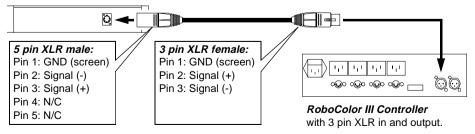
2 Connect the data output of the first *RoboColor III controller* to the data input of the next device. Use the XLR-XLR cable supplied when connecting to another RoboColor III controller or fixture with Martin polarity (pin 3 cold). Use a phase-reversing cable when connecting to a DMX device (pin 3 hot).
