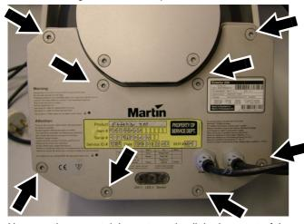
3. Unscrew the two retaining nuts and pull the base out of the casing, taking care not to stress any wire connections.
