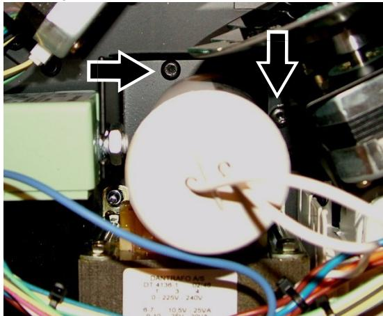
4. Use a wrench to remove the 13 mm capacitor retaining nut and lock washer to release the capacitor from the mounting bracket.
