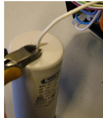
5. Use a wire cutter to clip the wires as close to the capacitor as possible.
