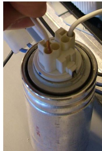
7. Press each end into a terminal on each side of the new capacitor to establish a circuit through the capacitor (the capacitor is not polarized).
