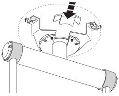
5 Move the Alien 02 Pendant to the correct pan position and screw the two pan locking screws in place using the 3 mm Allen wrench. Loosen the three Allen screws on the arms of the J-Box.
