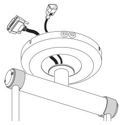
4 Slide the flange into the slot on the J-Box. Replace the slotted section (note that the dotted circle represents a cutaway of the J-box cover).
