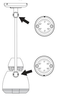
You can adjust the angle of the supporting arms, or the lamp, by making adjustments at the joints at two positions. To adjust a joint, use the 3 mm Allen wrench supplied with the fixture to loosen the joints on either side of the fixture. Adjust to the desired angle - +/- 50 degrees - and re-tighten.
