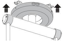
8 Using the 3 mm Allen wrench, tighten the three Allen screws that hold the cover in position.
