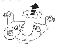
3 Pass the cables and mounting flange of the Alien 02 though the center of the J-Box cover.
