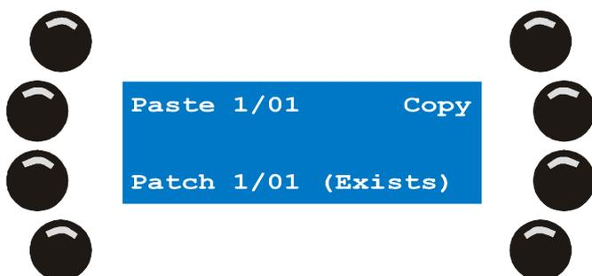
4. Use page keys 1-8 and general-purpose number keys 1-20 to select patch 102. In our example patch 102 is empty. Press {Paste 1/01} to paste the clipboard content into patch 102.
