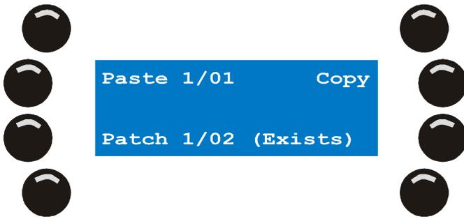
5. Press [ENT] to confirm and return to the patch menu. If you press [ESC] at this point, the patch is copied but not reloaded. The new patch still shows as empty until you exit and re-enter the patch menu.
