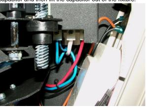
Replace the old capacitor with the new one, placing the capacitor back in the fixture and reconnecting the wires to both the capacitor and the starter.
