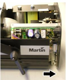
Use a wrench to remove the 13 mm capacitor retaining nut and lock washer to release the capacitor.
