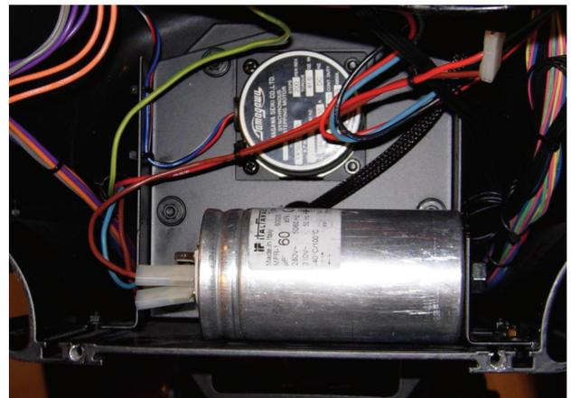
6. Check that all cables are still connected to the PCB, that all wires are in perfect condition and secured clear of moving parts, and that all connections are secure.
