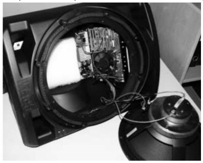
5 The jumper is located at the lower-right corner of the PCB. To enable the stand-by function remove the jumper at position JP1 (if present). To disable the stand-by function add a jumper (P/N 05120701).
