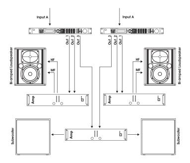
This example shows how 2 MACH M20.04s can be used in conjunction to distribute Input signals to a 3 or 4 way system per side.
