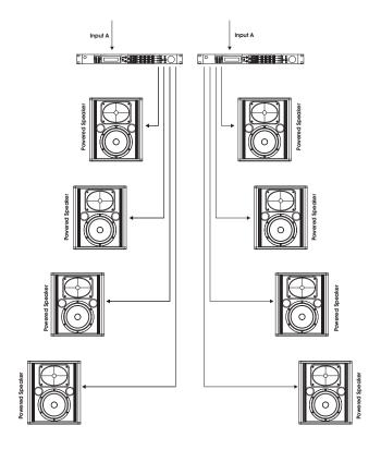
This example is similar to the previous example. However, the idea here is to distribute the signal with delay settings corresponding to the positioning of the speakers.
