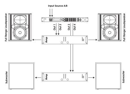
This is a typical stereo setup with a set of subs.
