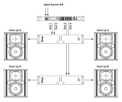
This setup is a typical small 2-way system.
