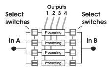
The Routing section is the "railway-station" in the signal chain. The signal present on Inputs A/B can via the 2x4 select switches be routed to none, any or all of the four Output channels.
