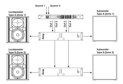
This setup is used where two different zones or rooms need to be covered. In this case Stereo is not the object.
