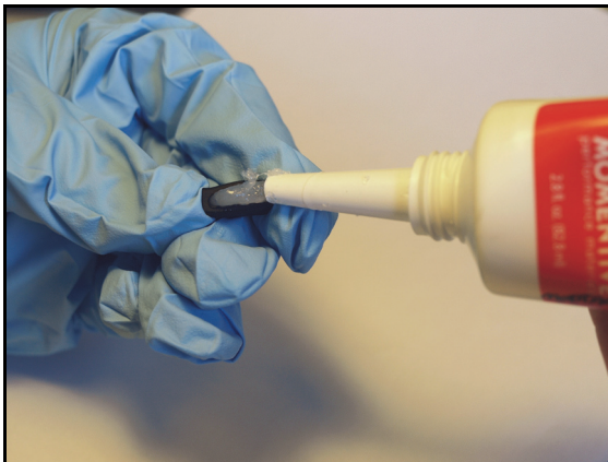
Figure 3. Applying sealant and installing a cap
