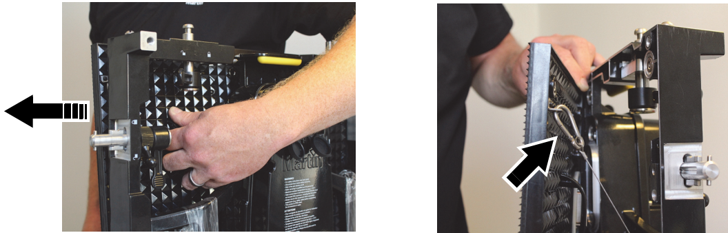
Figure 20: Replacing an LED block, rear access
