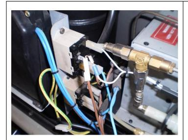
6. Connect Brown Wire 1 (with headers at both ends) to the piggy-back crimp and cover with the small piece of heatshrink.
