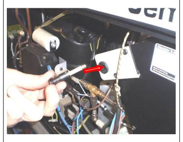
11. Insert fuse into Fuse Holder as shown.
