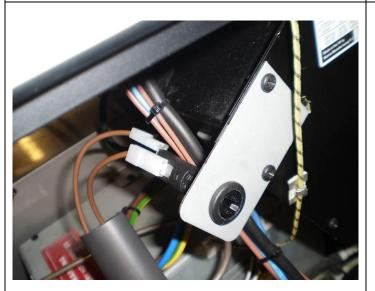
8. Connect the header of Brown Wire 2 (with red pin on end) to the top spade (which was bent in Step 2) on the Fuse Holder as shown and feed through the large piece of heat-shrink. Then feed the large piece of heat-shrink over the Fuse Holder.
