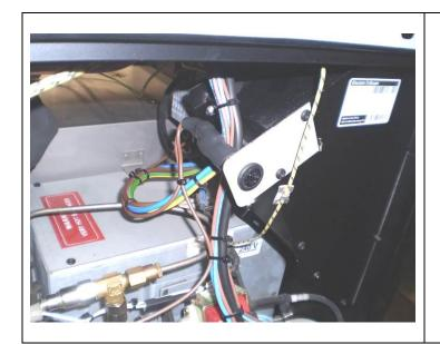
12. Finally, dress wires with cable ties.
