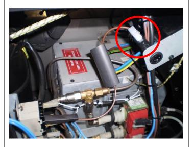
7. Feed through the large piece of heatshrink and connect to the outer pin of the Fuse Holder as shown.
