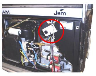
5. Fit the Fuse Plate assembly as shown using the 2 screws that were removed.
