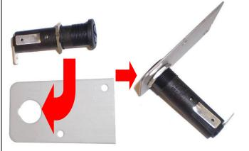
1. First, assemble Fuse Holder/Fuse Plate as shown by removing the silver nut, feeding the Fuse Holder into the fuse plate and finally securing with the silver nut.
