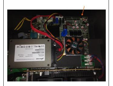
4. Locate Jumper "J\_ATXCTL1" on the mainboard (see arrow).
