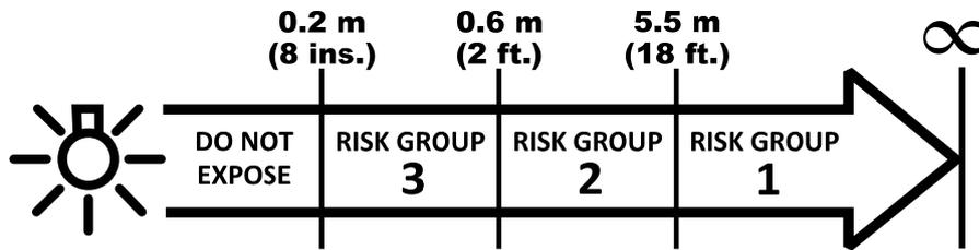
At a distance of less than 0.6 m (2 ft.) from the fixture, the light output can potentially cause eye or skin injury before an exposed person's natural aversion responses (blink reflex and reaction to skin discomfort) can protect them. At distances greater than 0.6 m (2 ft.), potential eye and skin injury hazards from the light output are normally prevented by natural aversion reflexes.
