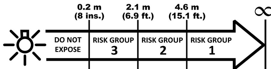
At a distance of less than 2.1 m (6.9 ft.) from the fixture, the light output can potentially cause eye or skin injury before an exposed person's natural aversion responses (blink reflex and reaction to skin discomfort) can protect them. At distances greater than 2.1 m (6.9 ft.), potential eye and skin injury hazards from the light output are normally prevented by natural aversion reflexes.
