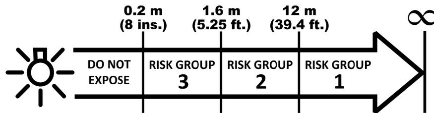
At a distance of less than 1.6 m (5.25 ft.) from the fixture, the light output can potentially cause eye or skin injury before an exposed person's natural aversion responses (blink reflex and reaction to skin discomfort) can protect them. At distances greater than 1.6 m (5.25 ft.), potential eye and skin injury hazards from the light output are normally prevented by natural aversion reflexes.
