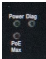
FIG. 16 System Status LEDs
