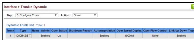
FIG. 73 Showing Connection Parameters for Dynamic Trunks
