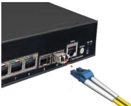
FIG. 15 Making a Connection to an SFP Port
