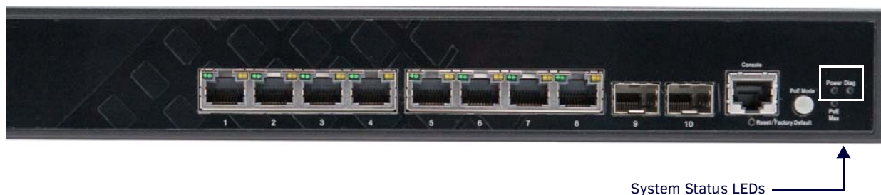
FIG. 4 System Status LEDs
