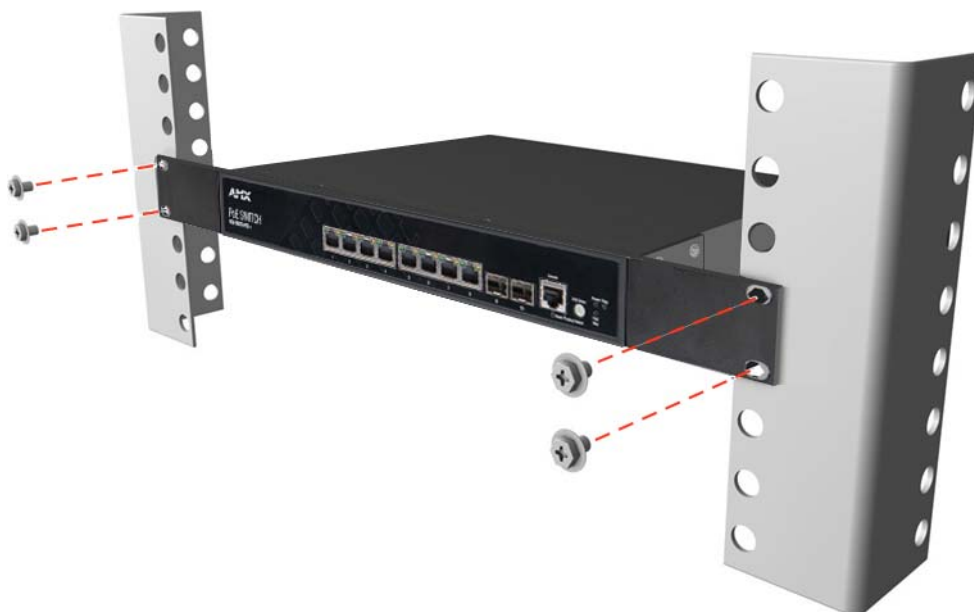
FIG. 2 Installing the Switch in a Rack
