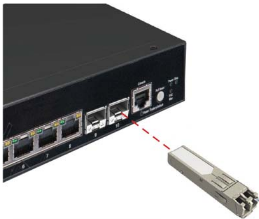
FIG. 13 Inserting an SFP Transceiver into a Slot
