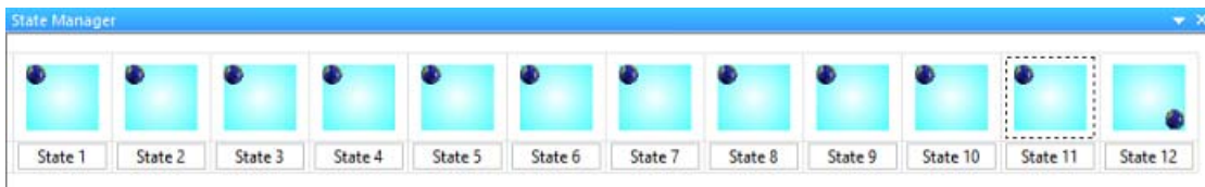
FIG. 326 State Manager window - multi-state button with 12 states with bitmaps
