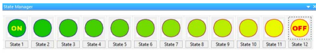
FIG. 313 State Manager window showing a button with 12 states and Tweened colors
