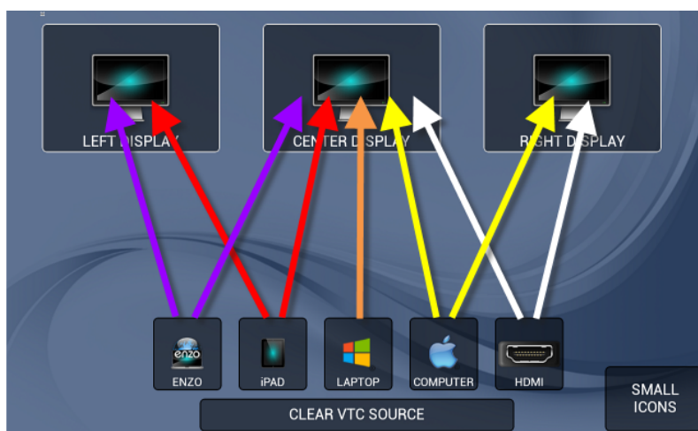
FIG. 271 Drop Target and Draggable Buttons - Drop Group assignments
