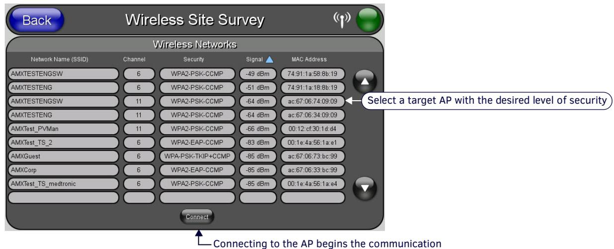
**FIG. 26** Site Survey of available APs (Secured AP shown selected)
