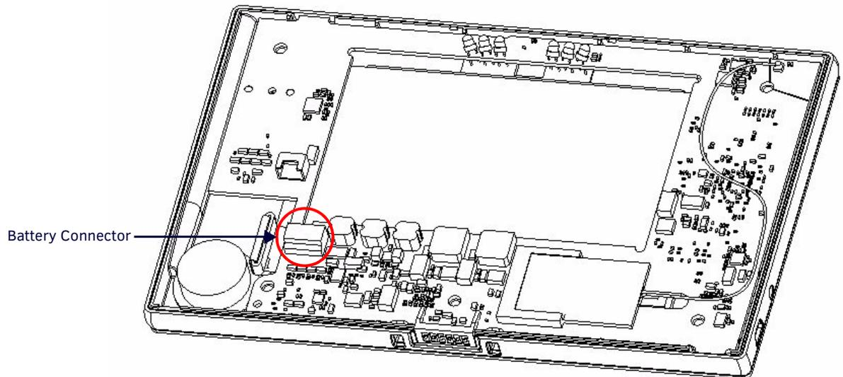
**FIG. 84** Battery installation and connection diagram
