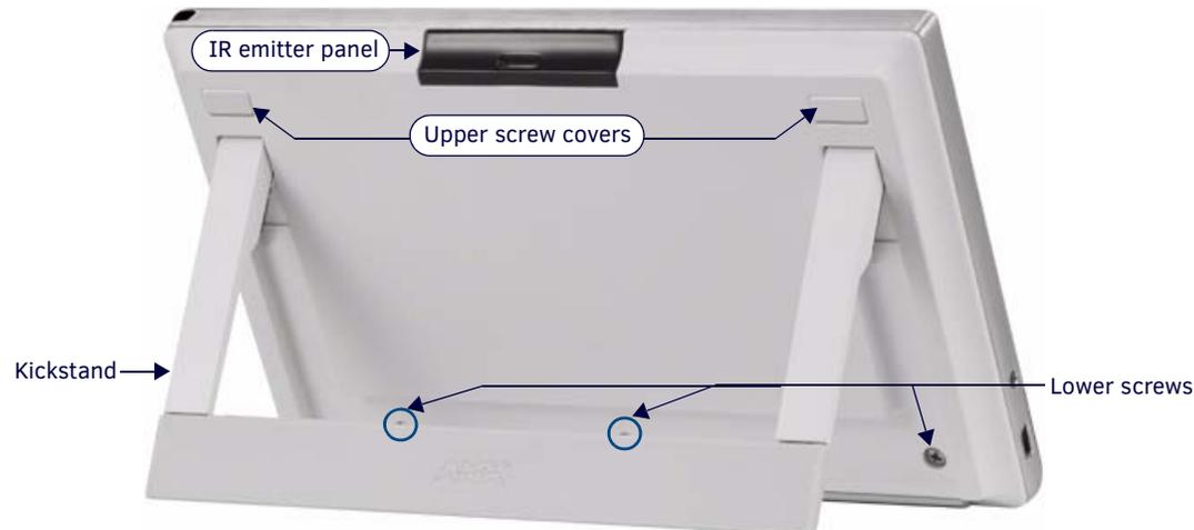
**FIG. 83** Screw placement at the back of the MVP-5200i- GW
