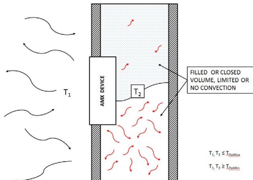
**FIG. 15** Heat convection in filled or closed volume, limited or no convection
