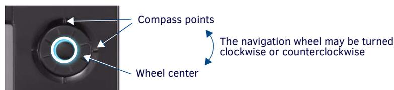
**FIG. 4** Navigation wheel detail
