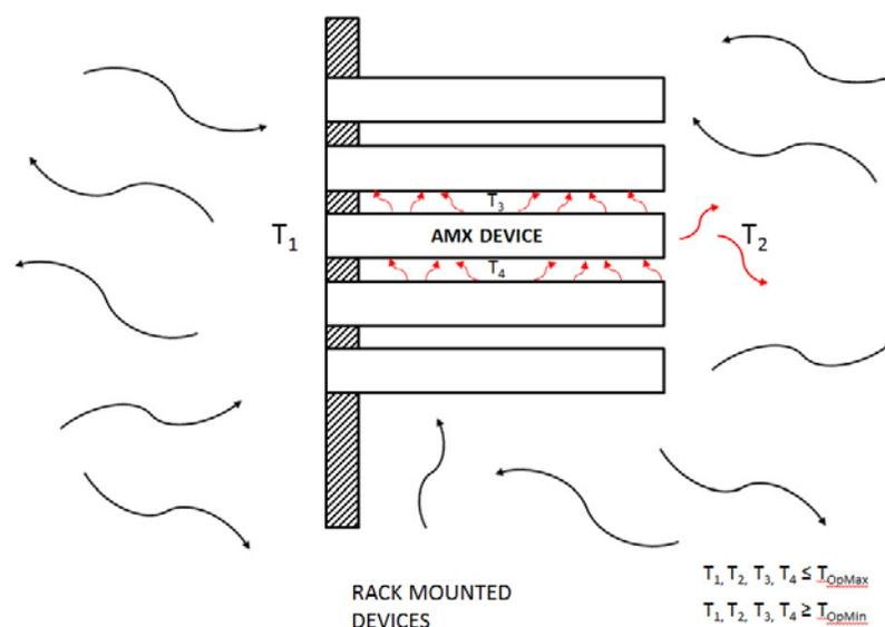
**FIG. 16** Heat convection in rack-mounted devices
