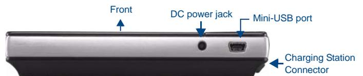
FIG. 2 MVP-5200i Connector Locations
