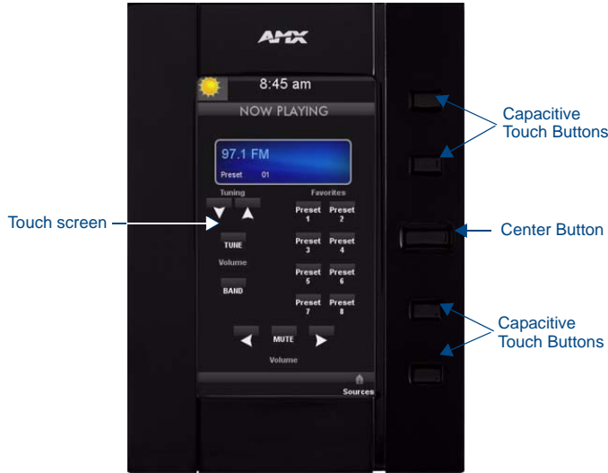
FIG. 1 NXD-435P-BL 4.3" Modero Wall/Flush Mount Touch Panel - Black
