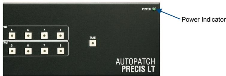
FIG. 22 Power indicator on control panel
