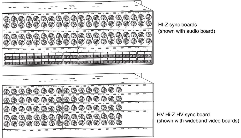
**FIG. 29** Hi-Z sync and HV Hi-Z sync boards
