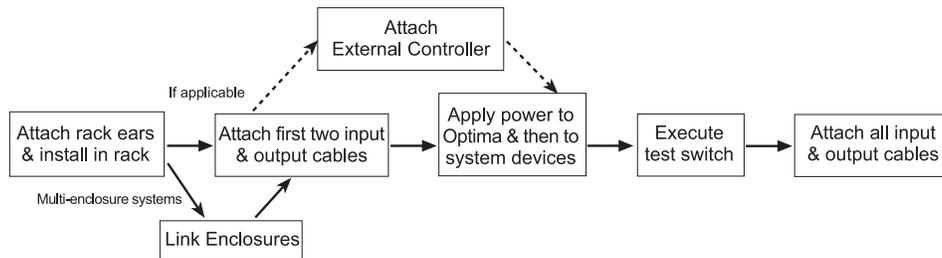
FIG. 7 Installation procedure
