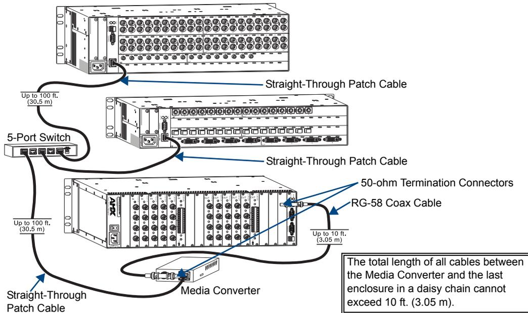
FIG. 12 Two Optima enclosures linked to a Modula enclosure
