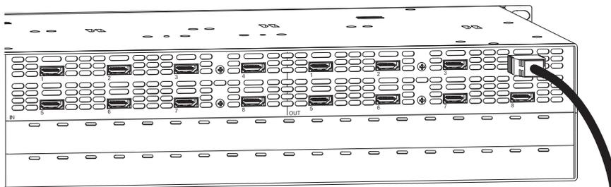
FIG. 42 Attach HDMI connectors to HDMI receptacles
