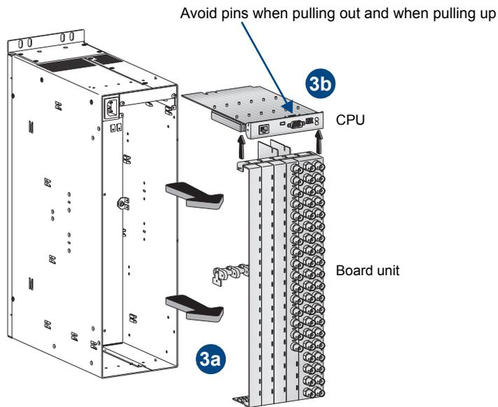
**FIG. 91** Pull CPU/board unit straight out and remove CPU
