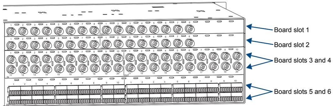
**FIG. 6** Input/output boards in an Optima 3 RU enclosure
