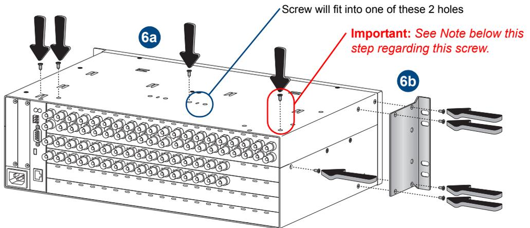
FIG. 100 Replace 5 screws and rack ear (4 screws)
