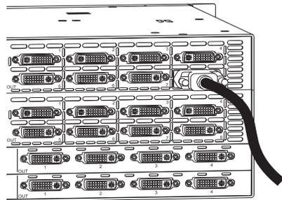
FIG. 39 Fasten cable onto the input or output DVI-I receptacle
