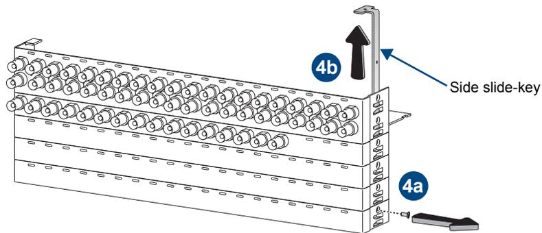
**FIG. 92** Remove side screw and slide-key
