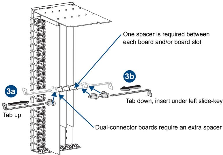
FIG. 97 Insert left and right slide-keys through spacers
