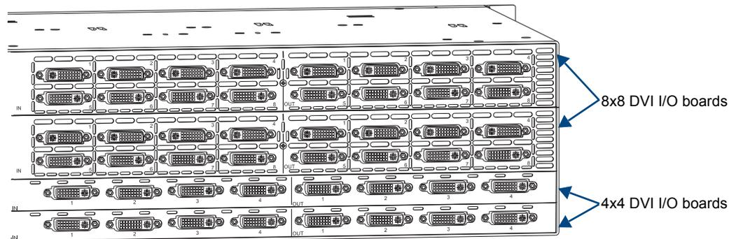
FIG. 37 Optima 8x8 and 4x4 DVI input/output boards
