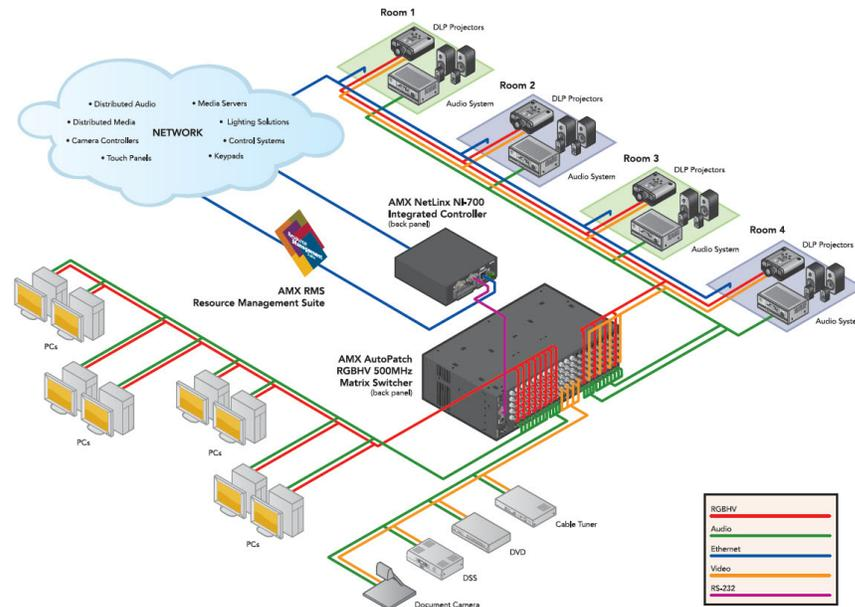
FIG. 1 System setup featuring the Optima Matrix Switcher
