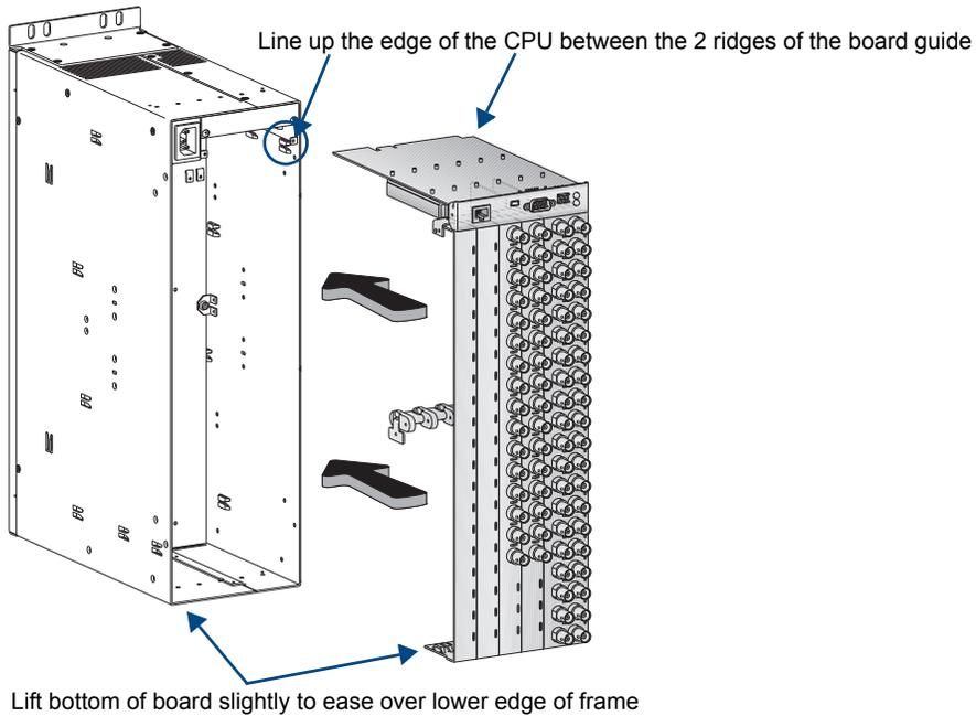
FIG. 98 Push CPU/board unit into place
