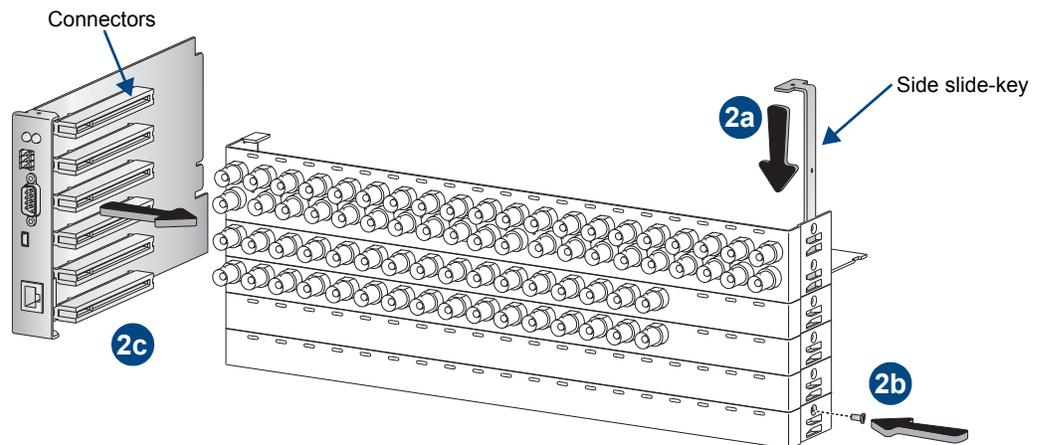
FIG. 96 Replace side slide-key and side screw; push board unit into place
