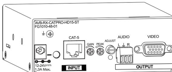
**FIG. 55** CatPro RGBHV+Stereo RX Module (rear view)
