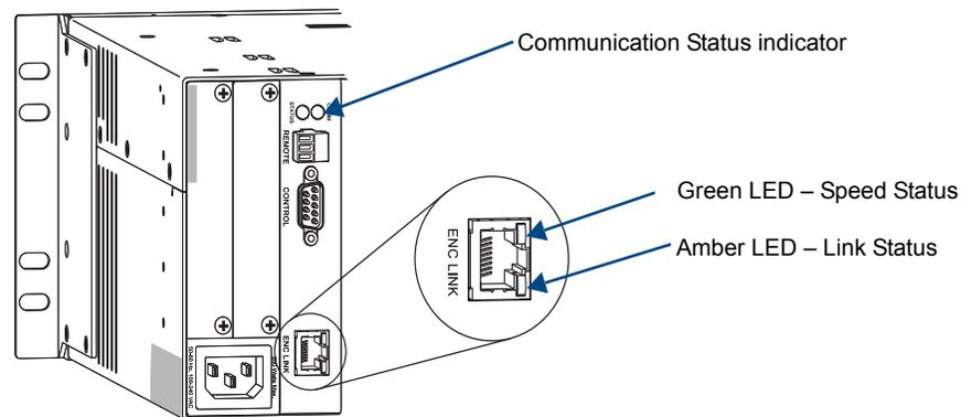
**FIG. 9** Ethernet connector LEDs
