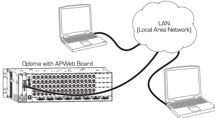
**FIG. 70** Optima enclosure with APWeb board connected to a LAN
