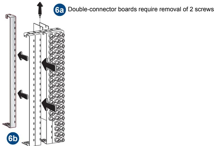
FIG. 94 Remove screw(s) and board or blank board plate
