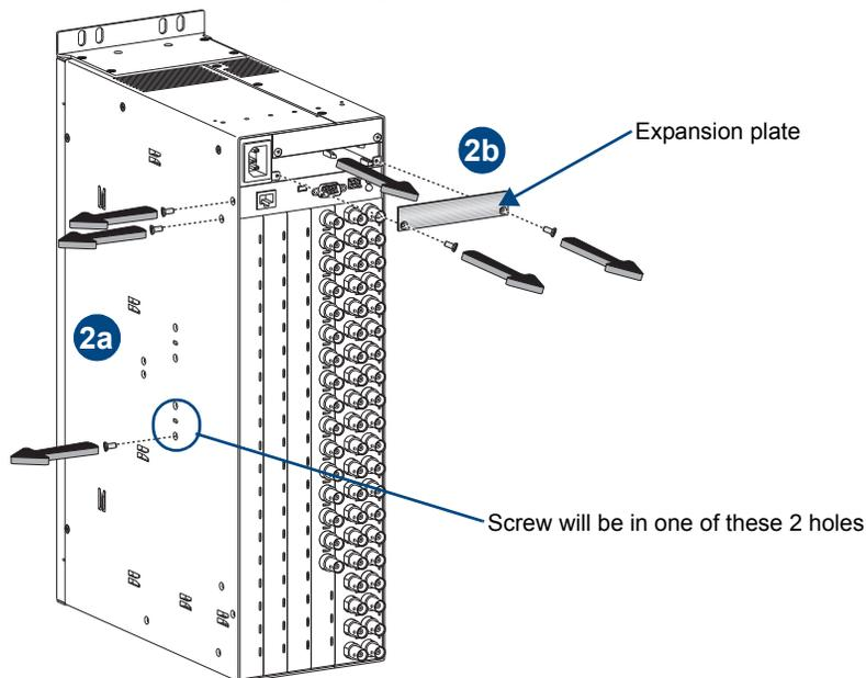
FIG. 90 Remove 3 screws and expansion plate (2 screws)
