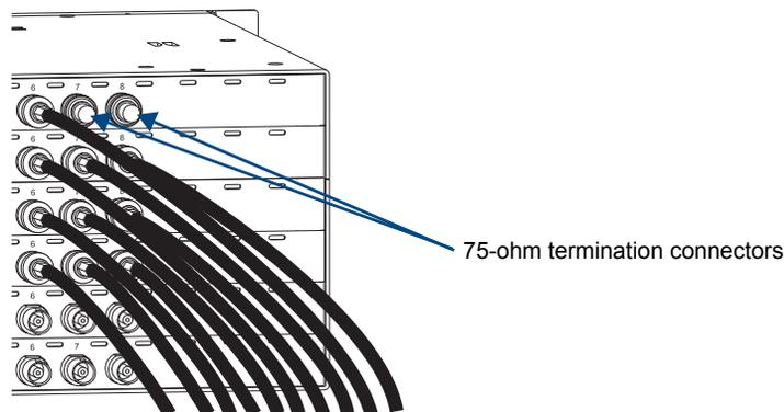
FIG. 36 Add 75-ohm termination connectors to unused outputs
