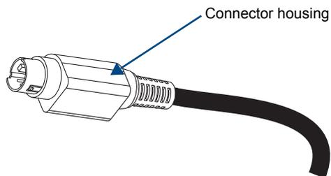
FIG. 24 Pull back housing to fasten the connector
