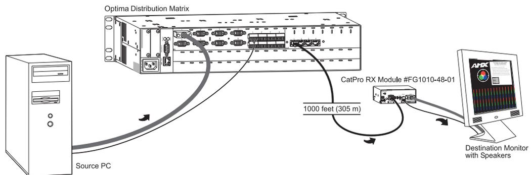
**FIG. 63** A typical Optima RGBHV+Stereo to CatPro system
