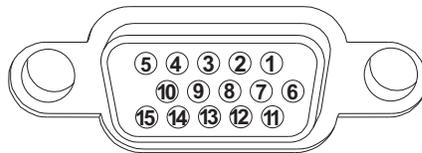
FIG. 33 RGBHV/HD-15 board connector pinout
