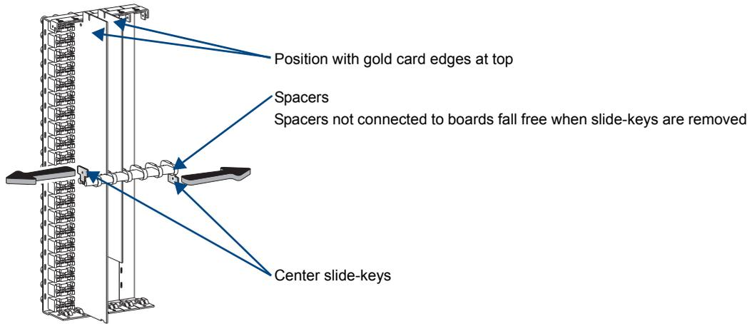
FIG. 93 Remove center slide-keys (2)
