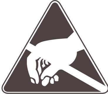
To avoid ESD (Electrostatic Discharge) damage to sensitive components, make sure you are properly grounded before touching any internal materials.
