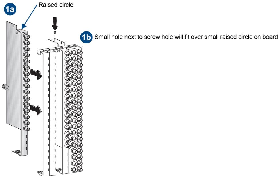
FIG. 95 Insert new board(s) and replace screw(s)
