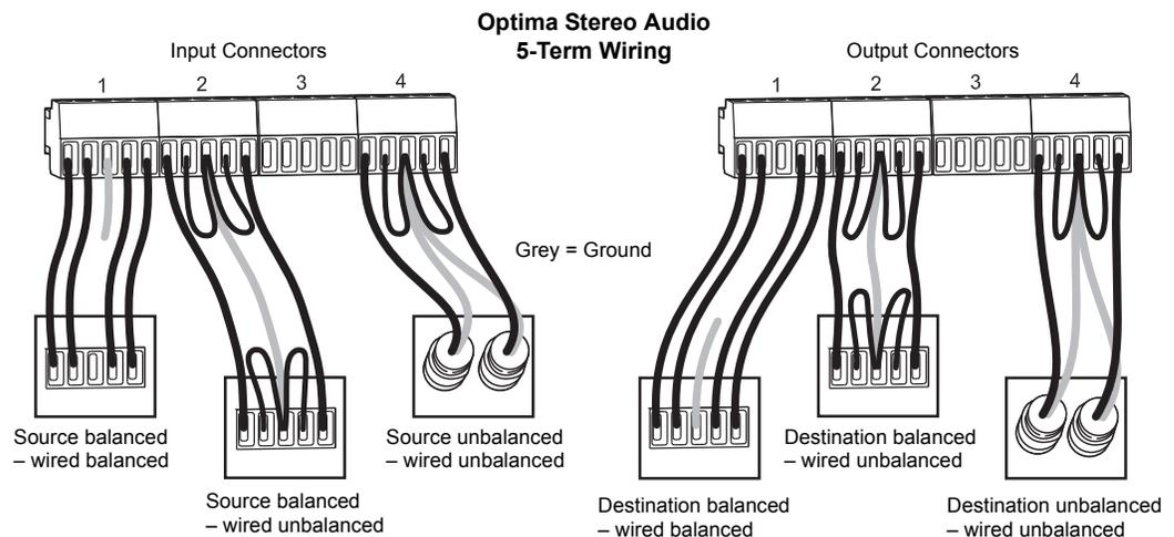
FIG. 53 Options for source-to-Optima-to-destination 5-term wiring
