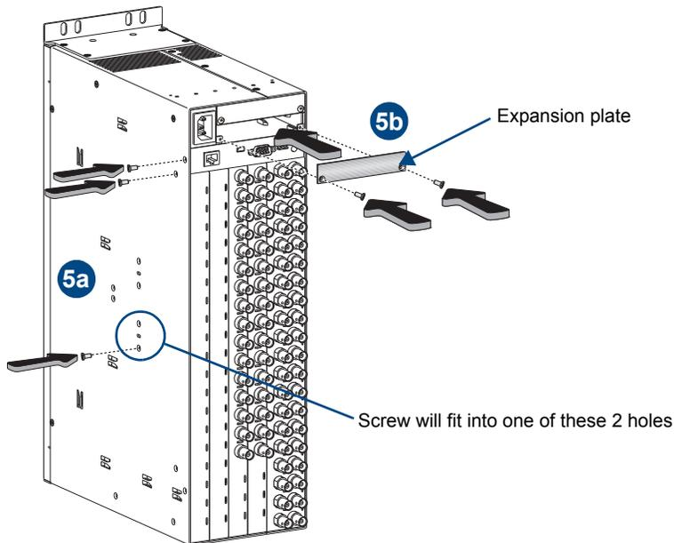
FIG. 99 Replace 3 screws and expansion plate (2 screws)
