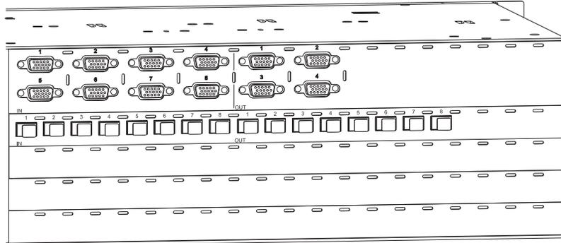
**FIG. 31** 8x4 RGBHV/HD-15 I/O board (shown with an 8x8 digital audio board)
