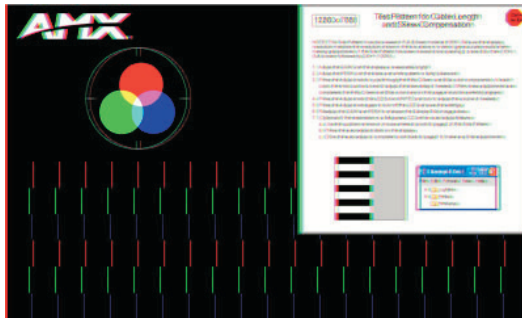
FIG. 49 Test image adjusted for gain and peak (image is still skewed)
