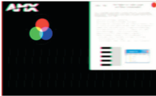
FIG. 52 Test image on Destination Monitor with distorted display
