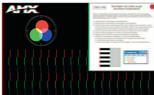
FIG. 54 Test image adjusted for gain and peak (image is still skewed)
