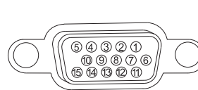
FIG. 5 HD-15 (board) connector pinout
