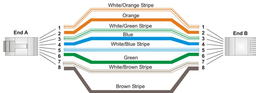
FIG. 11 RJ-45 wiring diagram
