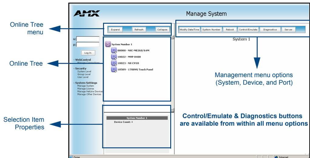
**FIG. 43** System Settings - Manage System page
