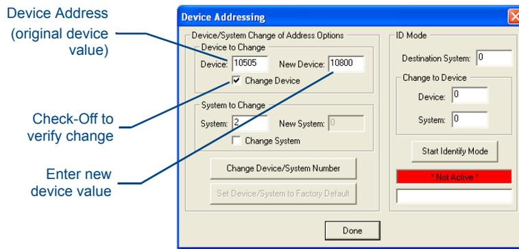
FIG. 17 Device Addressing dialog (changing the device value)
