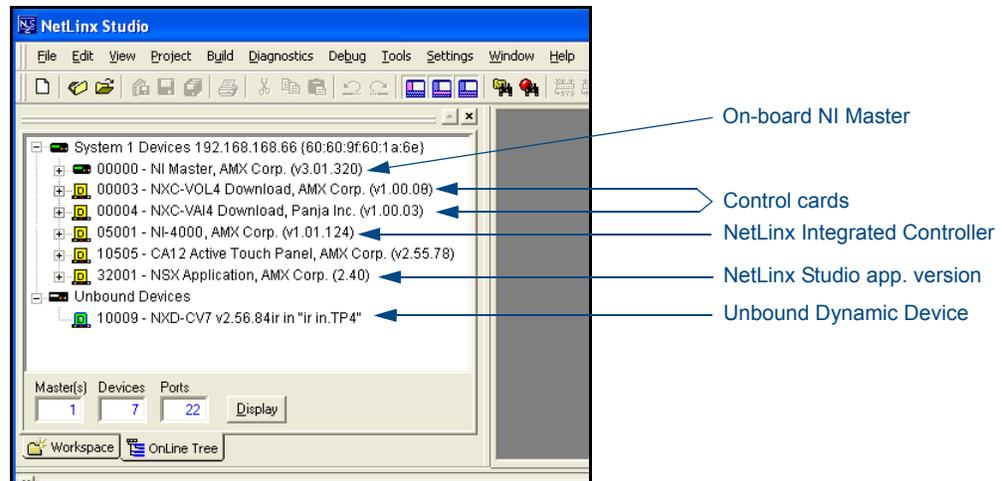
FIG. 28 Sample NetLinx Workspace window (showing OnLine Tree tab)
