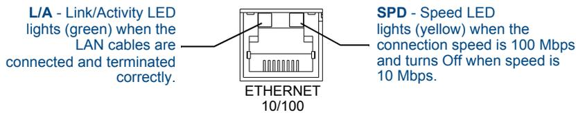
FIG. 12 LAN LEDs
