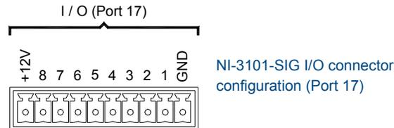
FIG. 9 INPUT/OUTPUT connector (male)
