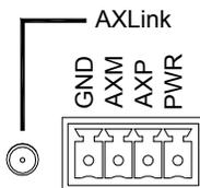
FIG. 3 AXlink connector and LED
