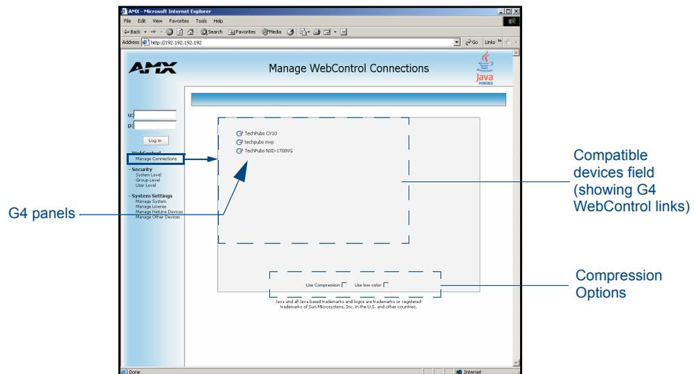
FIG. 34 Manage WebControl Connections page (populated with compatible panels)
