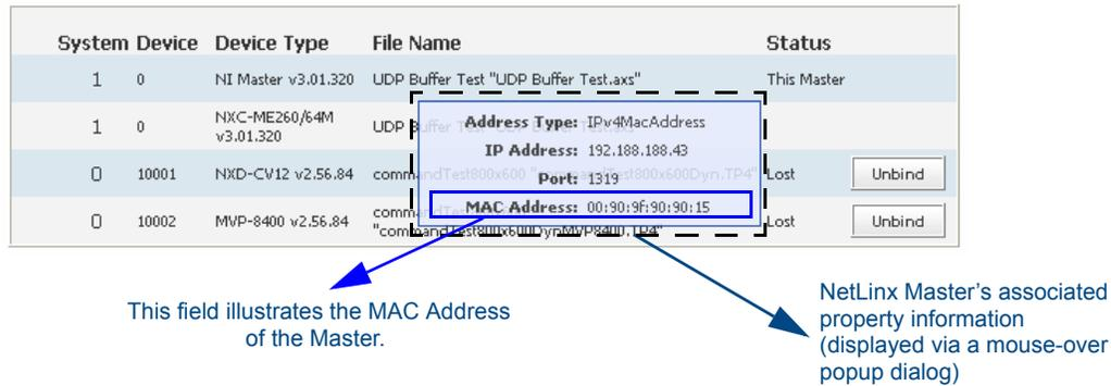
FIG. 63 Manage NetLinX Devices page - showing a sample mouse-over popup dialog
