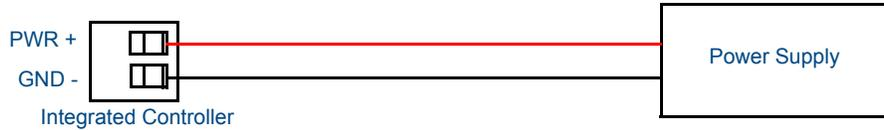
**FIG. 4** 2-pin mini-Phoenix connector wiring diagram (direct power)
