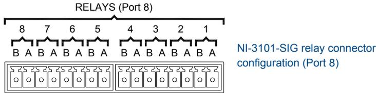
FIG. 8 RELAY connector (male) NI-3101-SIG
