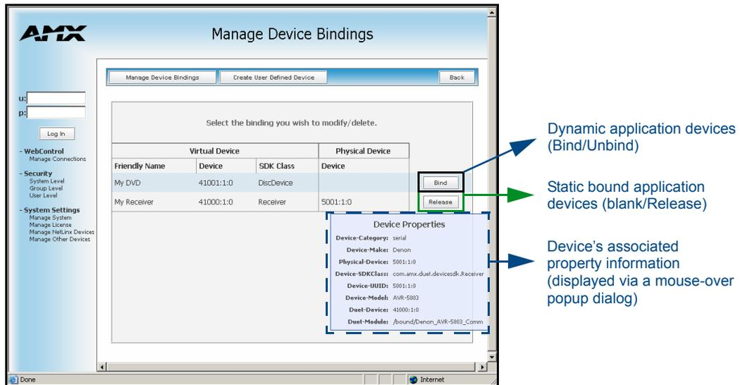
**FIG. 68** Manage Device Bindings page
