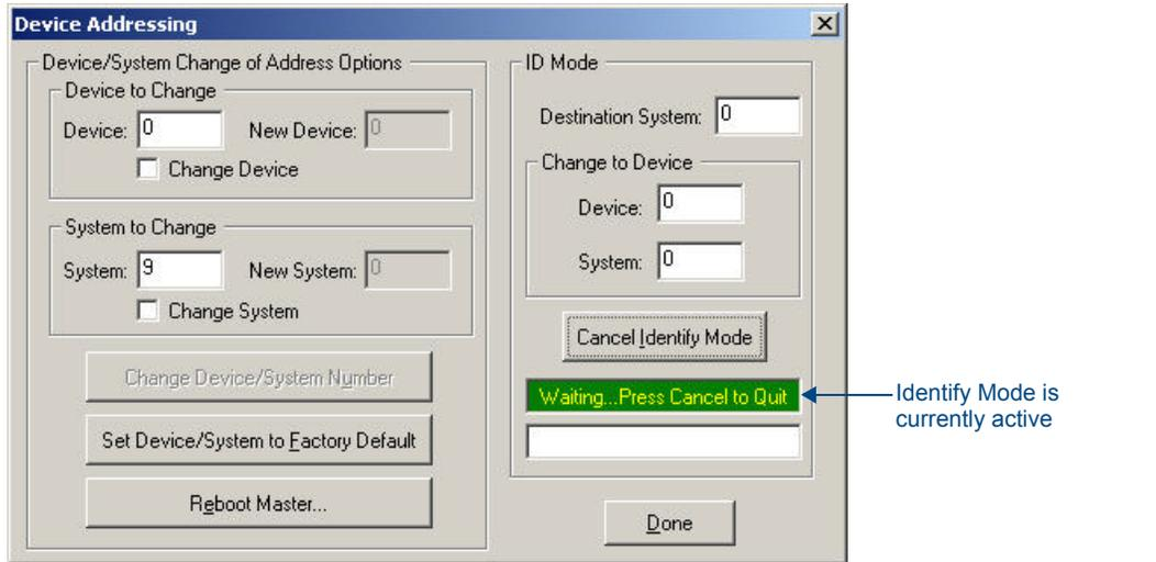
FIG. 19 Device Addressing dialog - Identify Mode active
