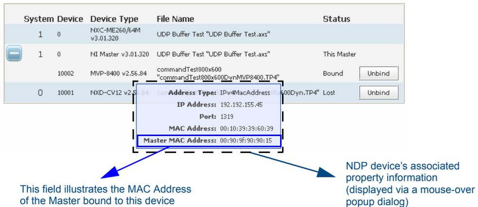
FIG. 64 Manage NetLinX Devices page - showing a sample mouse-over popup dialog
